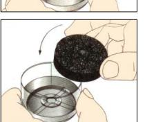
4. Insert the displacer piston spring and center it in the bottom of the lower part of the can.
