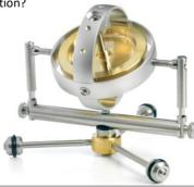
Using the same configuration as configuration 2 but using one or two of the extension rods that come with the gyroscope, screw them into one of the threaded holes of the gyroscope. Spin the gyroscope up using the electric motor and lift the extension rods up like shown in the picture. Let go and watch what happens. The gyroscope will slowly precess around.
