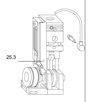
The sparkplug should be checked through the carburettor opening because the sparkplug is no longer tight if the plastic part is repeatedly unscrewed.
