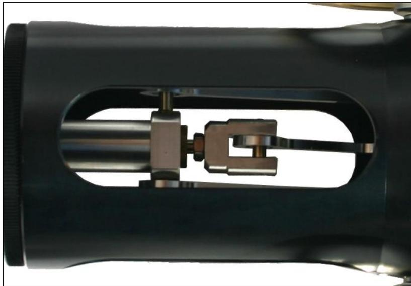
1. Undo nut the shown in the centre of the picture above (only one or two turns to loosen)
